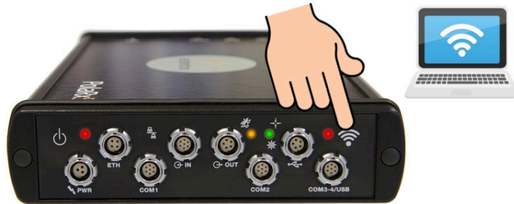
Figure 3-6: Press firmly on the front-panel WiFi button to turn on the WiFi modem. When active, the red WiFi led will be lit.
