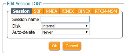
Figure 4-28: Select 'External' from the drop-down list to log data to an external memory device
