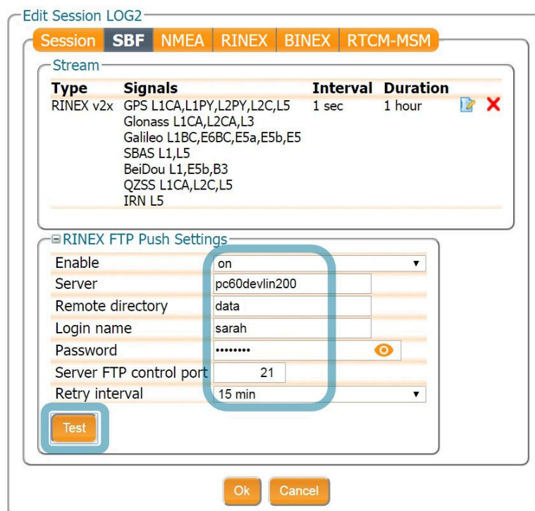
Figure 4-29: Configure pushing of RINEX files to an external FTP server
