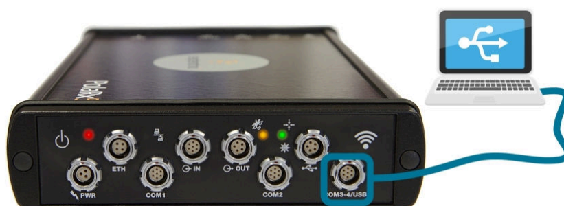
Figure 3-3: Connecting to the front-panel USB socket
